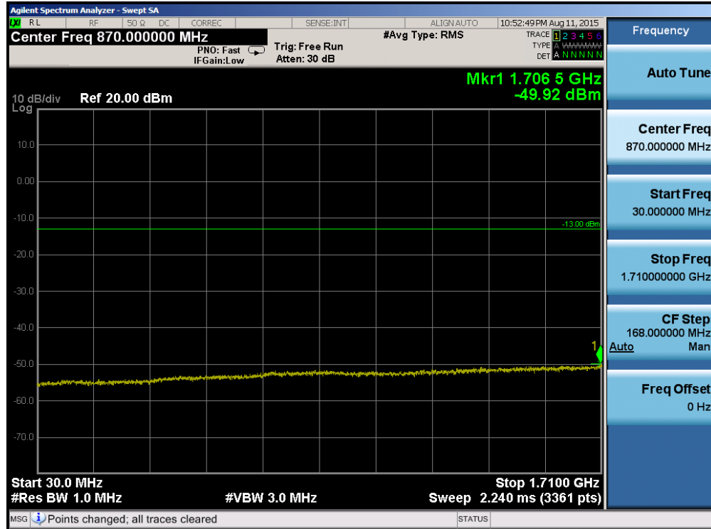
Plot 6-23. Conducted Spurious Plot (Band 4 – 5.0MHz QPSK – RB Size 1, RB Offset 0 – Mid Channel)
