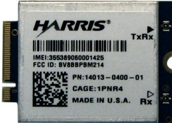
The label is 1.25" x 1.0" mylar with acrylic adhesive backing. The label is permanently attached to the metal shield on the LTE module during the manufacturing process in the orientation as shown in the photo above.
