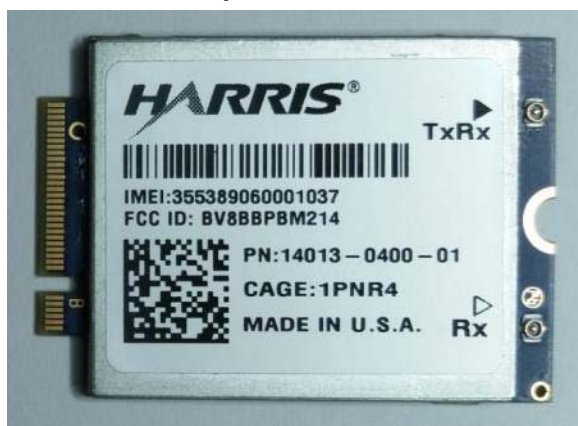
Module topside with shield
