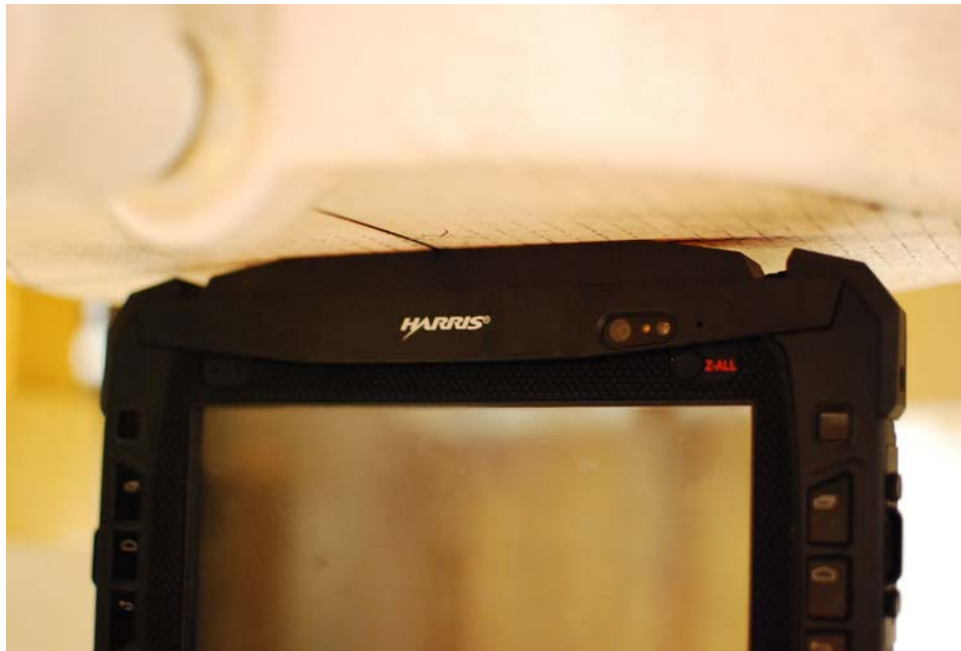
SAR Test Setup Photo 2: Top at 0.0 cm
