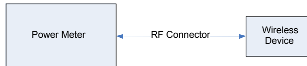
Figure 8-1 Power Measurement Setup
