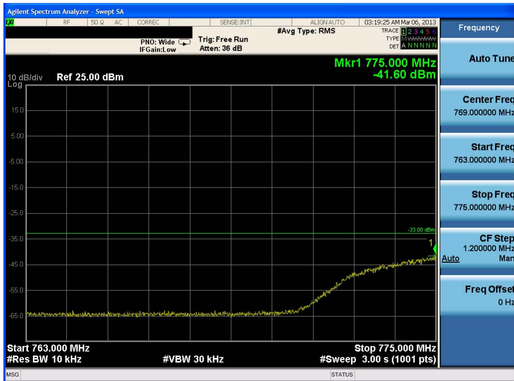
Plot 7-4. Lower Emission Mask Plot (16QAM, 50RB)
