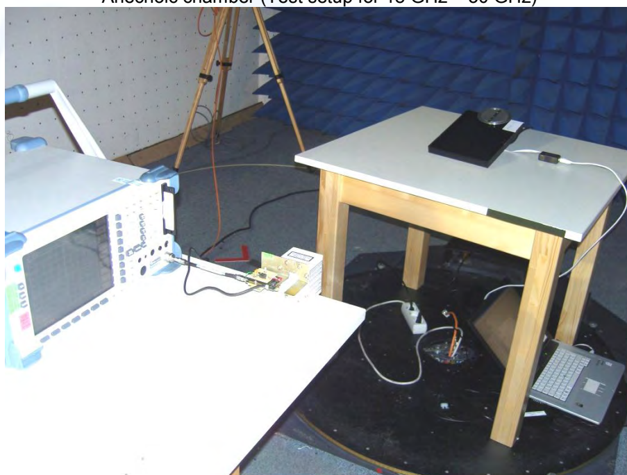
Anechoic chamber (Test setup for 18 GHz – 30 GHz)
