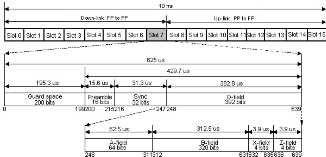
The basic, repeating, frame structure is 10 ms long. It is sub-divided into 16 slots, each 625  $\mu$ s long. The active transmission time is 429.7  $\mu$ s. The first 8 slots form the 'down-link', when the FP transmits to the PPs. The last 8 slots form the 'up-link', when the PPs transmit to the FP.
