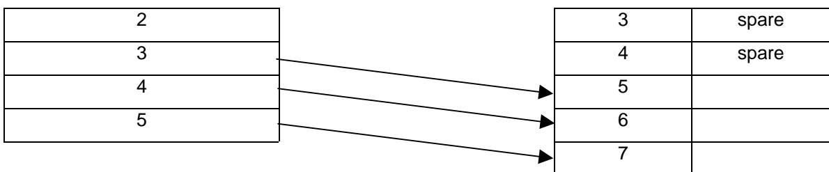
Noisy channels can be adapted out of the sequence by 'channel swapping', *i.e.* swapping a good spare channel for a noisy channel. For example, swapping physical channels 1 and 3 gives:
