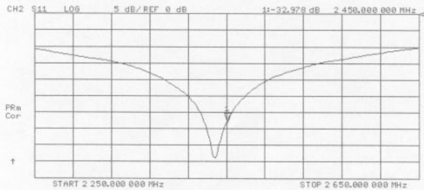
**Validation Dipole D2450V2 SN709, d = 10 mm**
