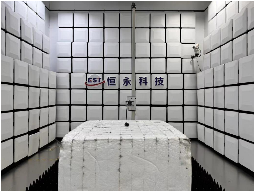
Radiated Test (Above 1GHz)
