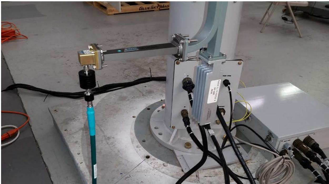
**FIELD STRENGTH SPURIOUS EMISSIONS FINAL SETUP**
