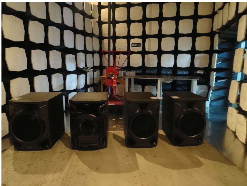
Photograph 2: Set-up for Spurious Emissions (30MHz-1GHz)
