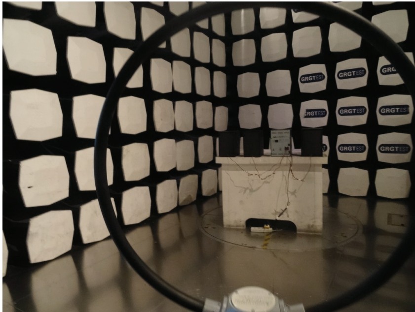
Photograph 2: Set-up for Spurious Emissions (30MHz-1GHz)
