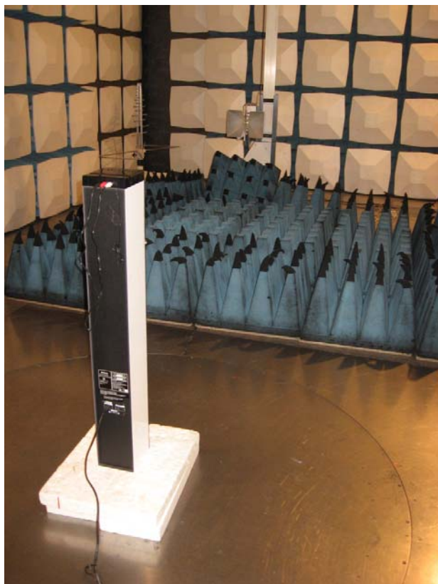
Photograph 3: Set-up for Radiation Measurement above 1GHz
