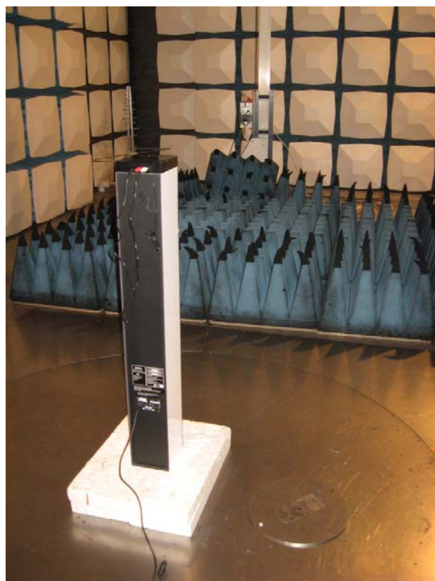
Photograph 3: Set-up for Radiation Measurement above 1GHz
