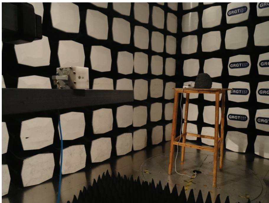
Photograph 2: Set-up for Spurious Emissions (above 1GHz)
