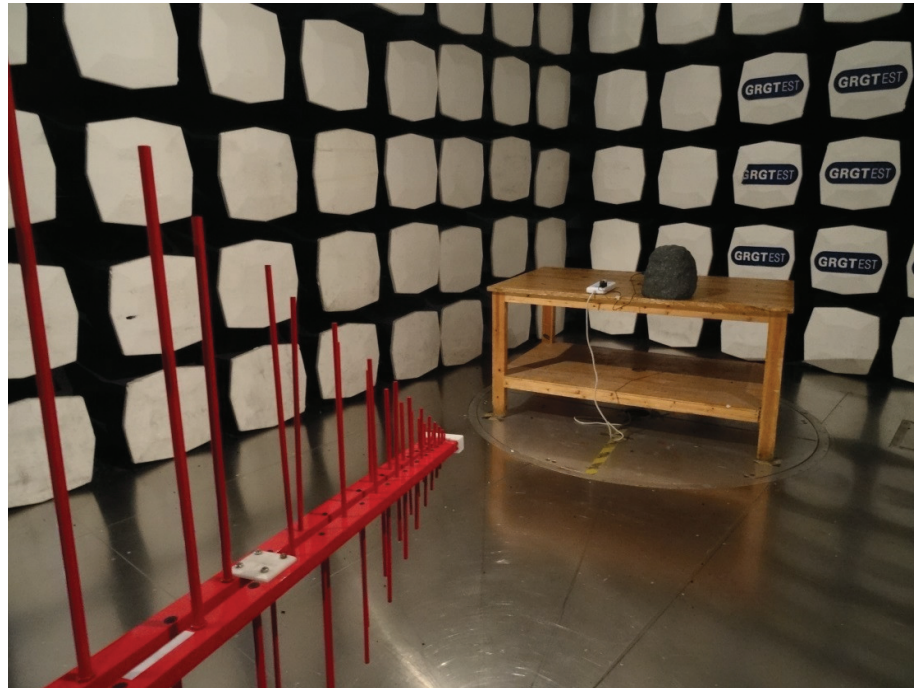
Photograph 2: Set-up for Spurious Emissions (above 1GHz)
