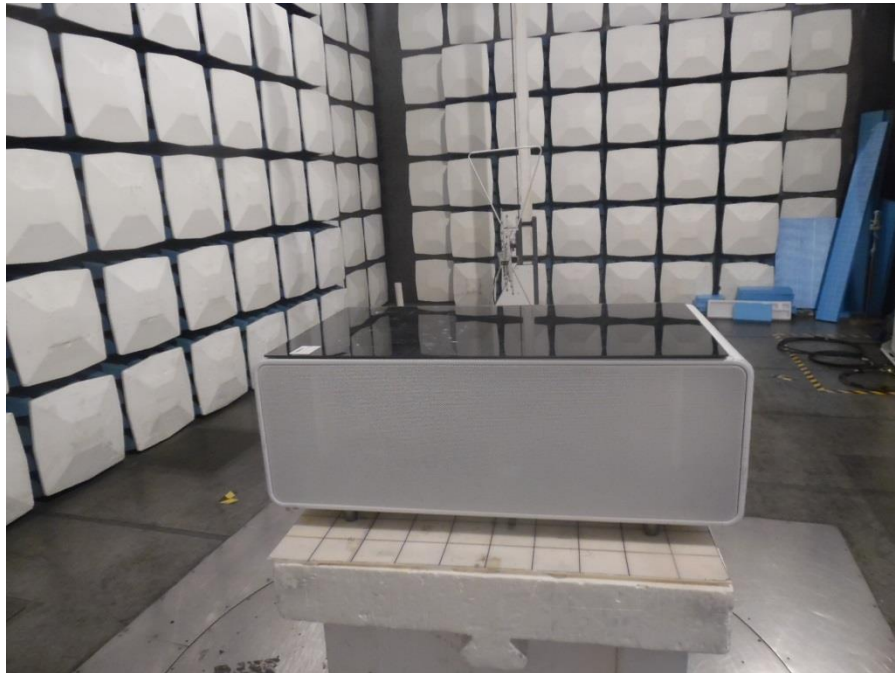
Photograph 2: Set-up for Spurious Emissions (above 1GHz)
