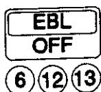
There are two EBLs (Electronic Bearing Lines). A numeric display of the positions of the EBLs is given, together with a rectangular highlight indicating which EBL can be adjusted via the EBL/DATA control.
