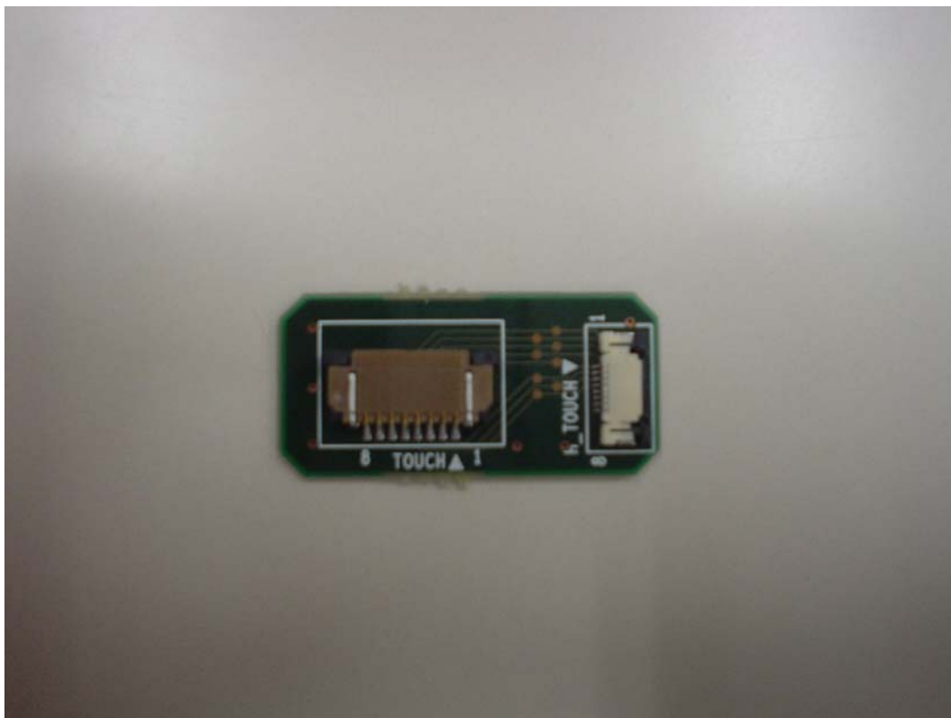
Touch Panel Connection Board (Front)
