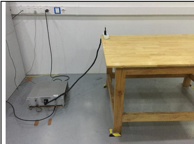
Conducted Emissions Test Setup – Front View
