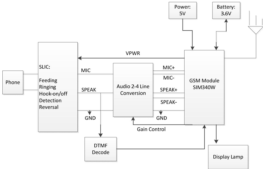
The power management network converts the 12V input from DC adaptor to 5V, Power supply to module, battery and system.
