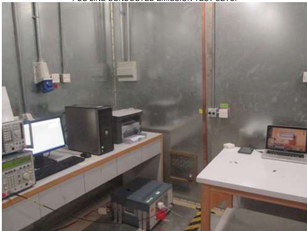
FCC RADIATED EMISSION TEST SETUP
