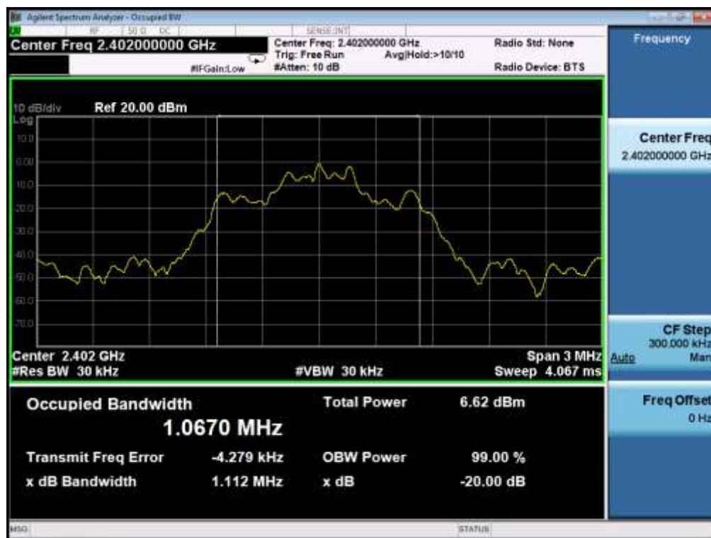
TEST PLOT OF BANDWIDTH FOR LOW CHANNEL
