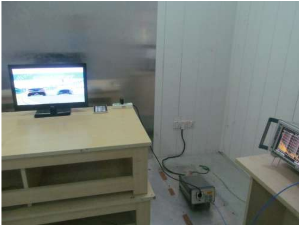
FCC RADIATED EMISSION TEST SETUP
