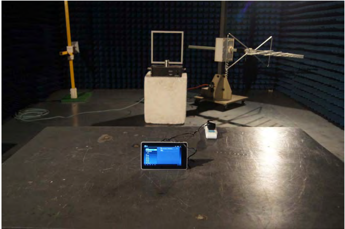
Radiated emissions test 30MHz- 1GHz
