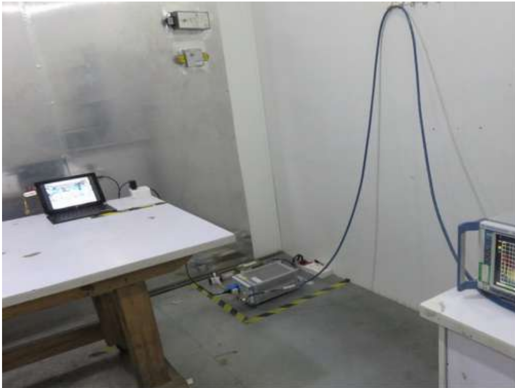
FCC RADIATED EMISSION TEST SETUP
