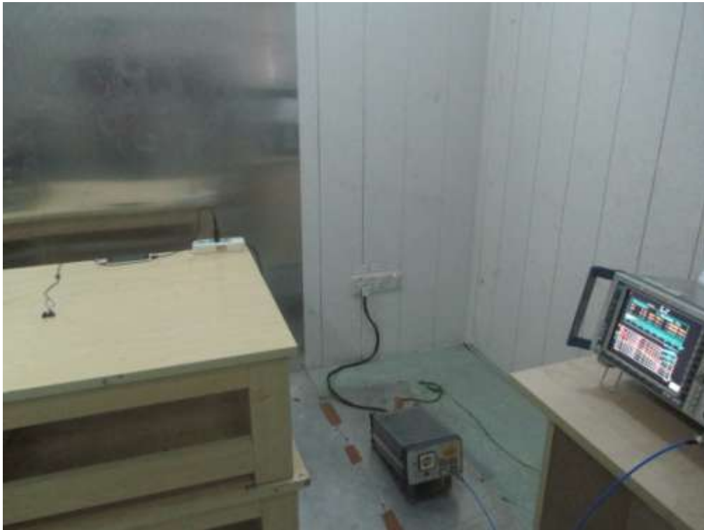
FCC RADIATED EMISSION TEST SETUP
