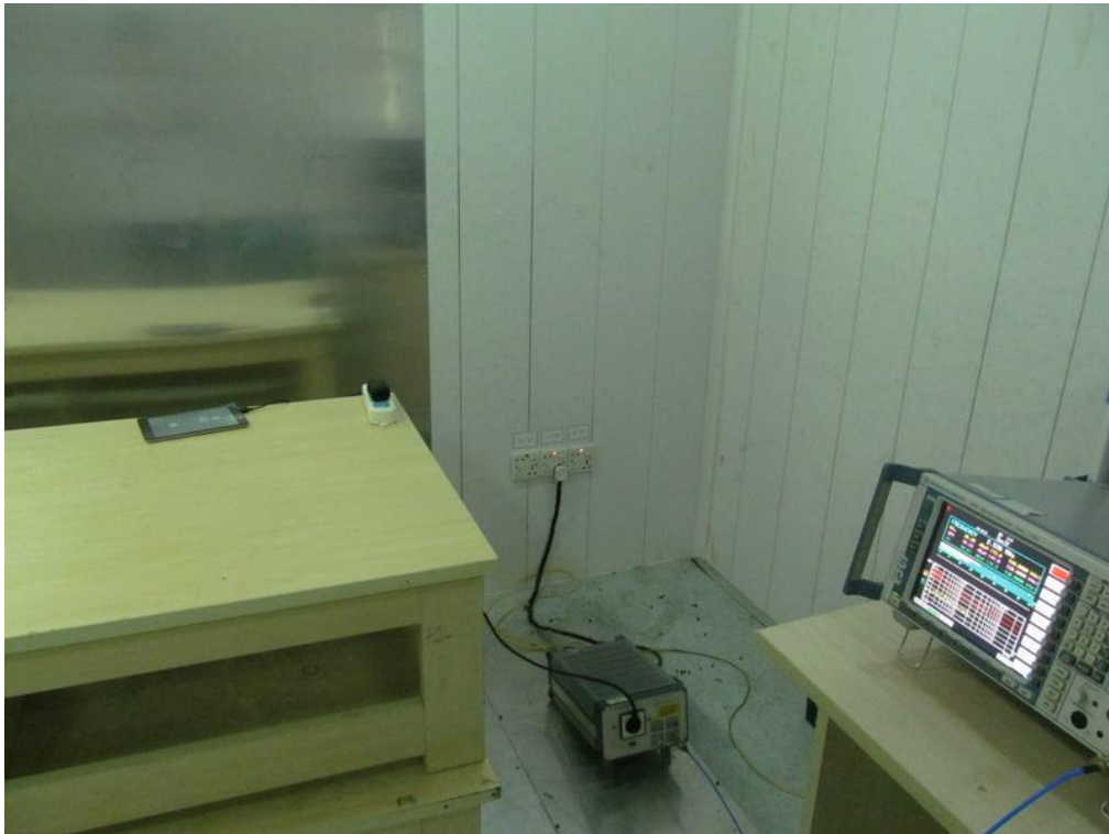
FCC RADIATED EMISSION TEST SETUP
