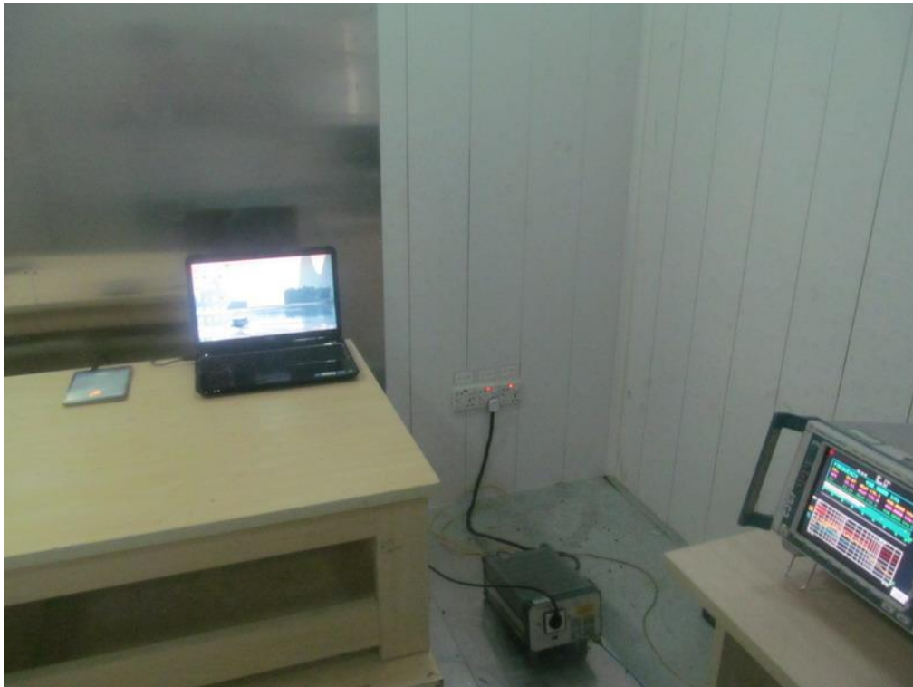
FCC RADIATED EMISSION TEST SETUP
