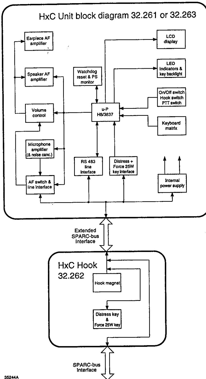
A handset unit contains two printed circuit boards: A board placed inside the handset (shown in the HXC unit block diagram above), and a board placed in the hook (shown in the HXC hook block diagram above). The handset hook board functions as an interface board between the handset extended SPARC-bus interface and the SPARC-bus interface.
