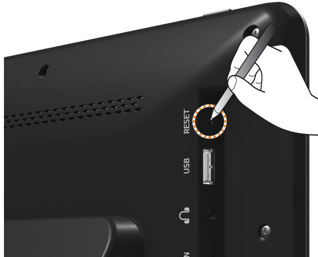
To reset the system, use a clip or a pin to press into the RESET button.
