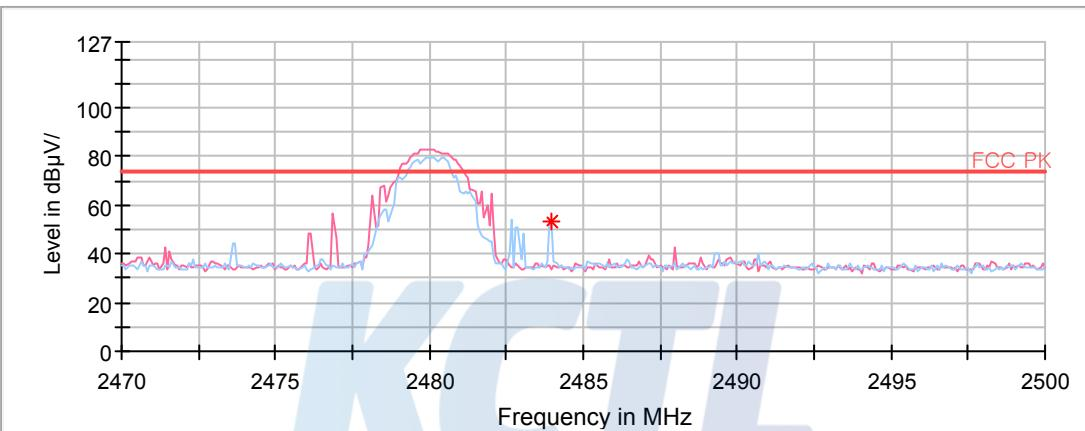
Note. DH5 & 3DH5 for testing, According to the formula, VBW was selected 500 Hz.
