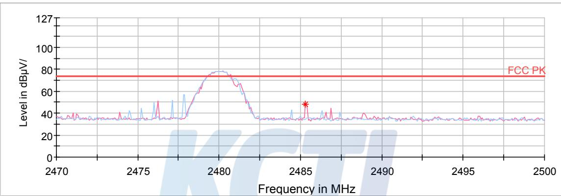
Note. DH5 & 3DH5 for testing, According to the formula, VBW was selected 500 Hz.
