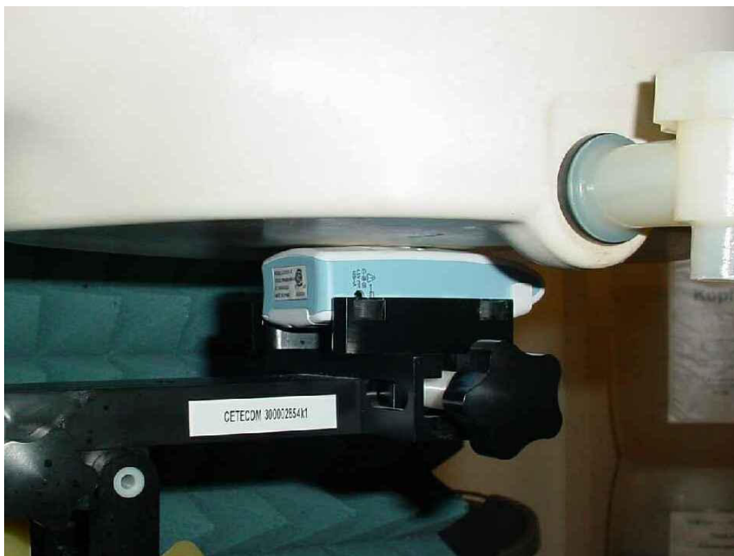
Photo 12: Test position body worn front side without any distance
