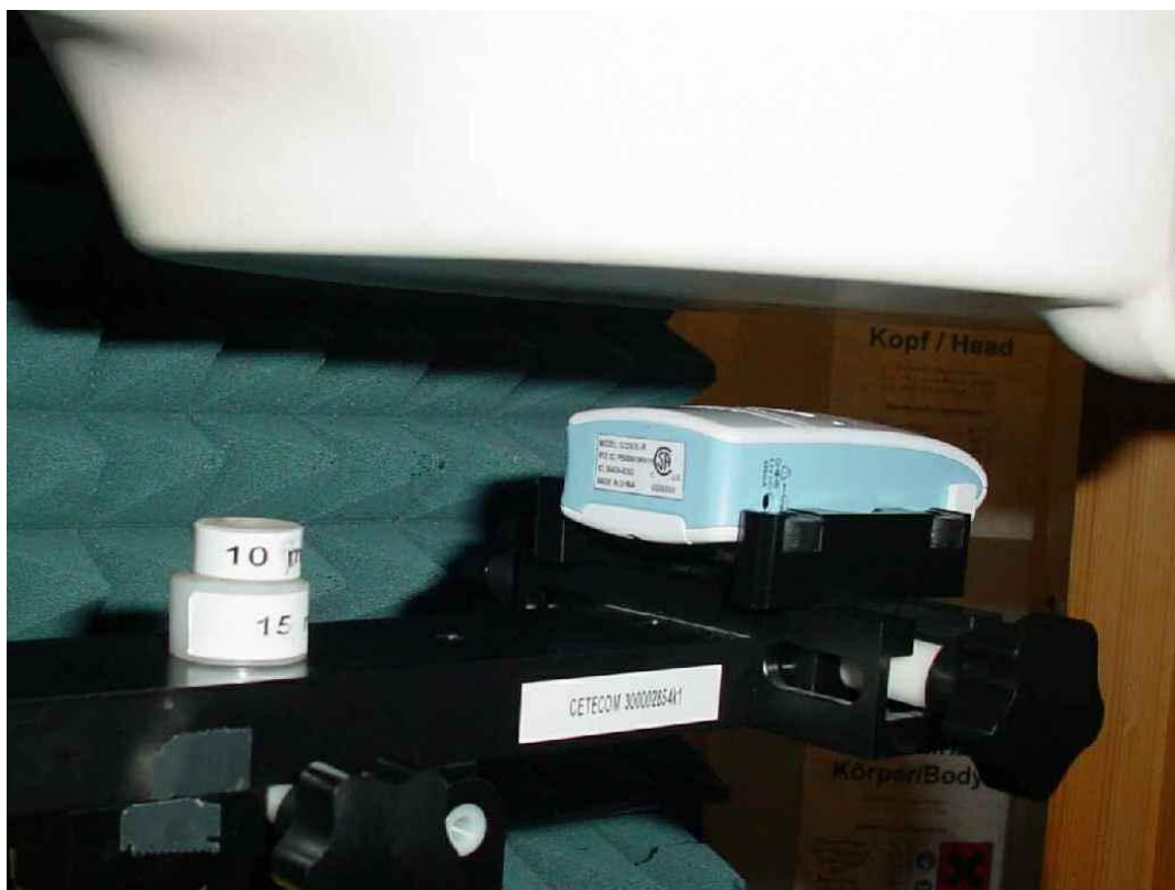
Photo 10: Test position front side with 25 mm distance
