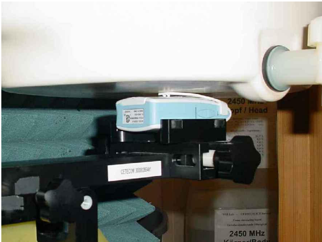
Photo 14: Test position body worn rear side without any distance
