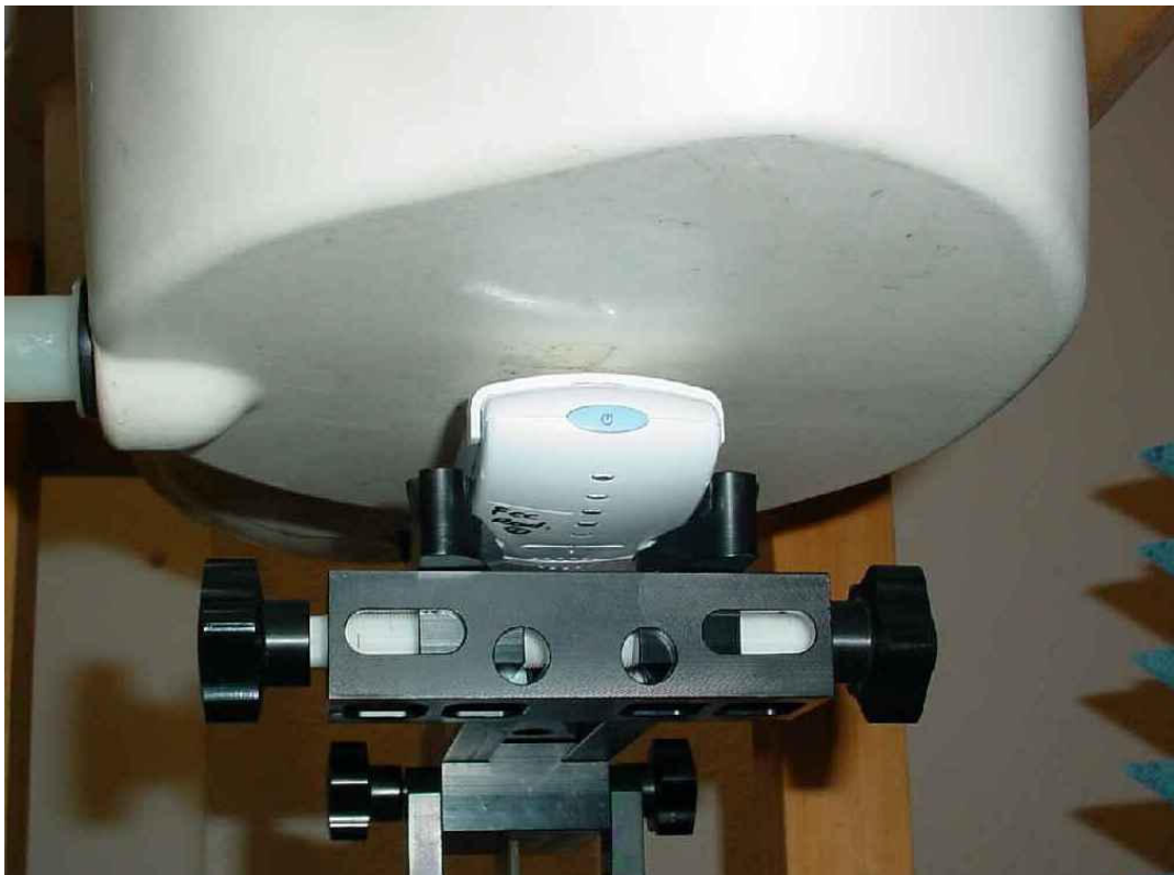
Photo 14: Test position body worn rear side without any distance
