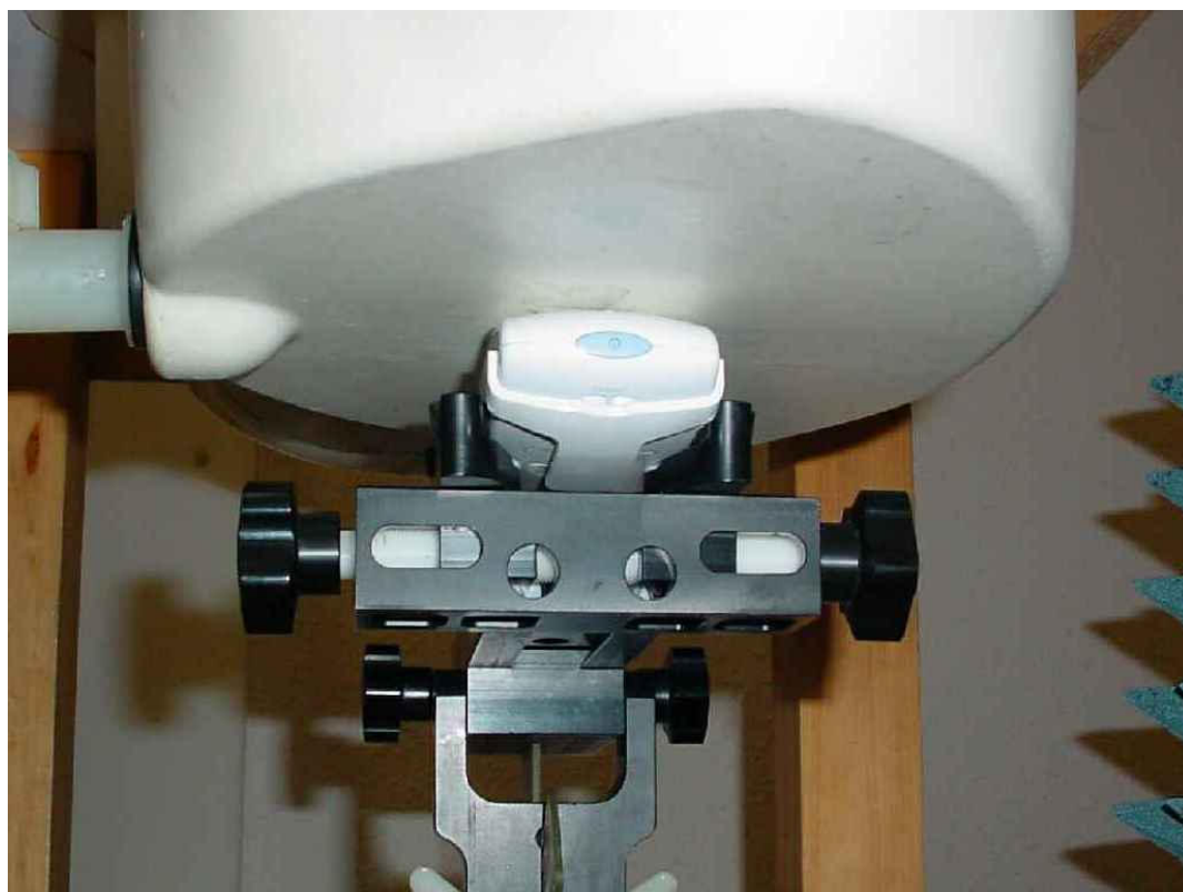
Photo 12: Test position body worn front side without any distance
