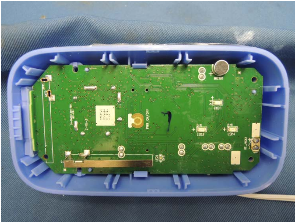
Baby Unit Main PCB solder side
