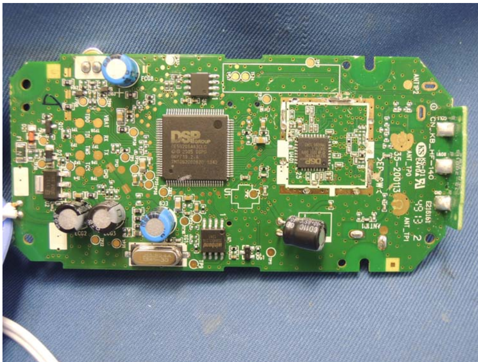
Baby Unit Main PCB comp side
