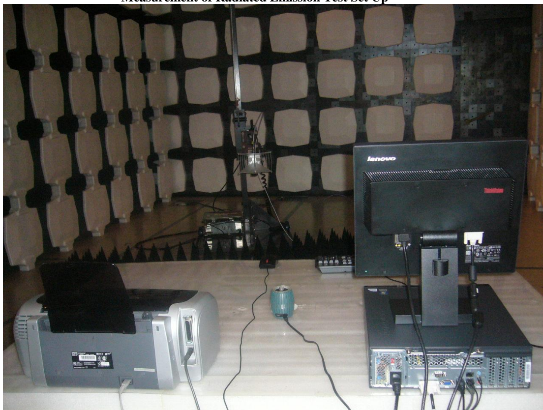
Measurement of Radiated Emission Test Set Up
