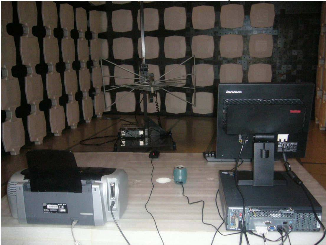
Measurement of Radiated Emission Test Set Up
