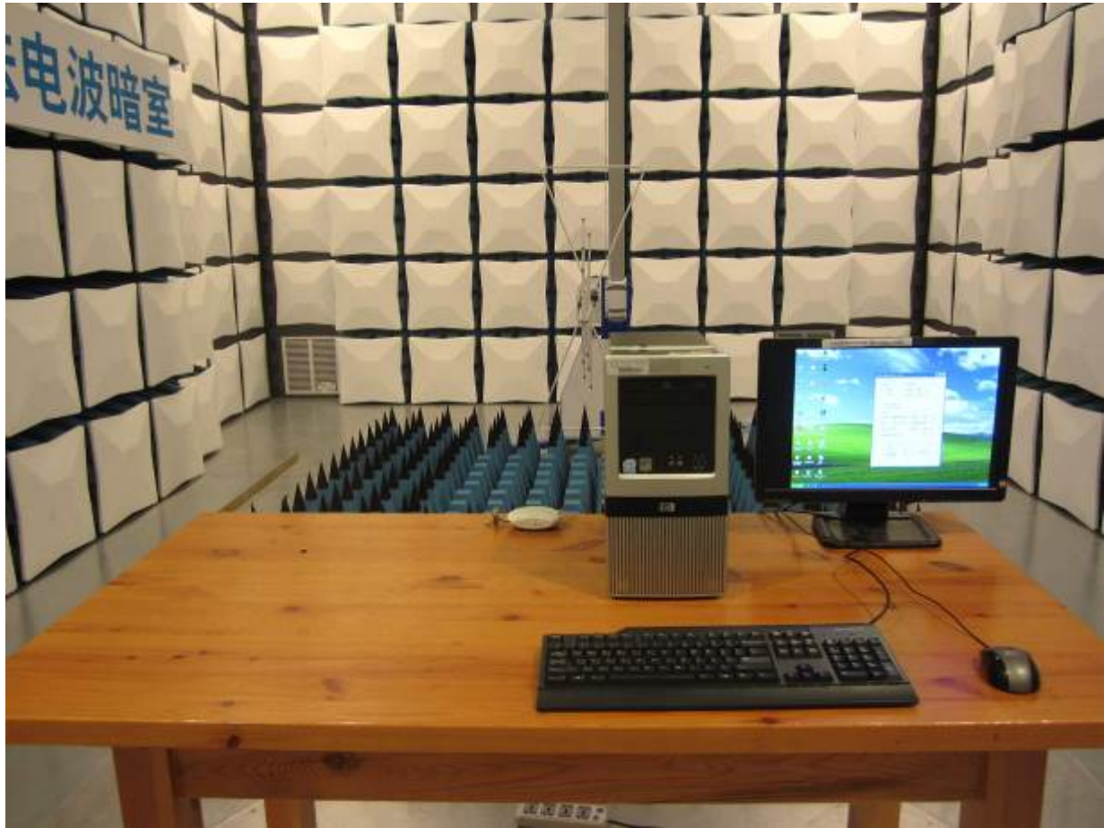
Figure 4 Radiated emission test setup (above 1 GHz)
