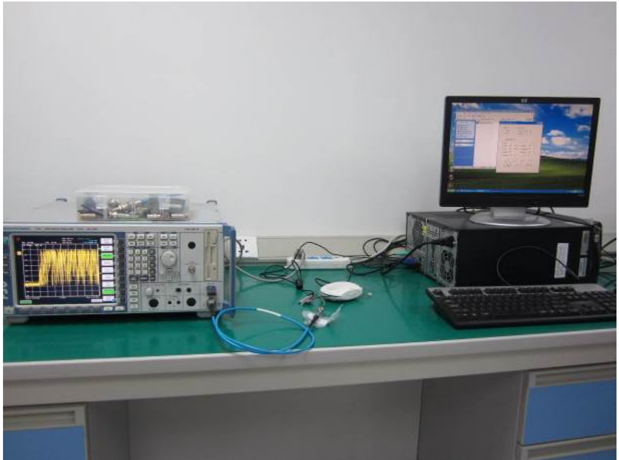
Figure 2 Conducted measurement Test setup
