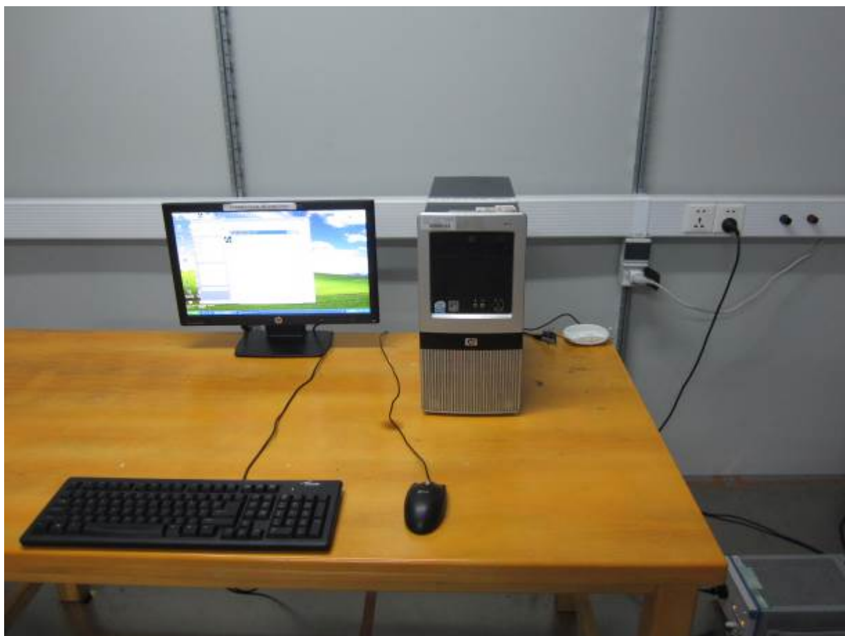
Figure 3 Conducted Emission test setup
