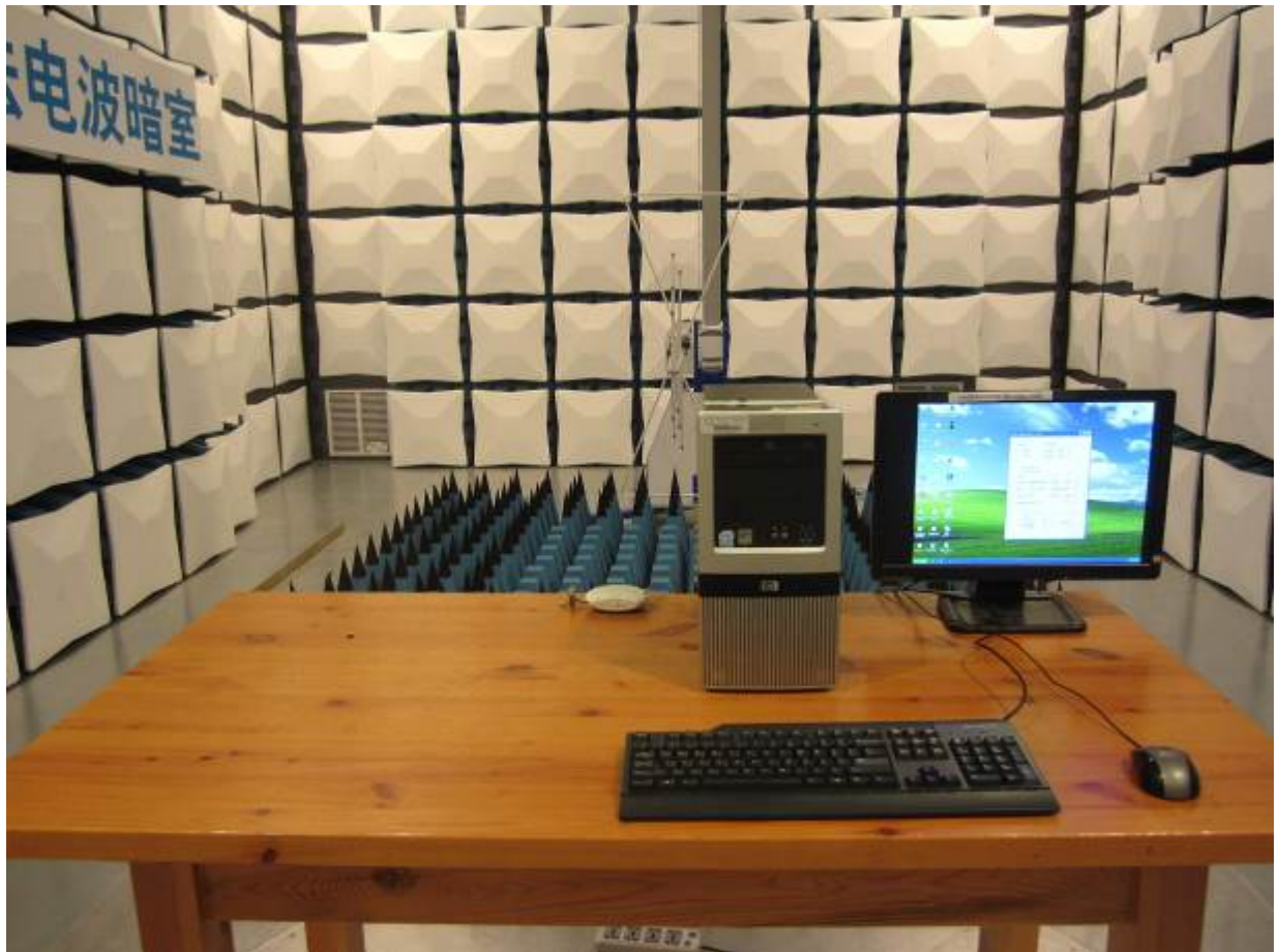
Figure 5 Radiated emission test setup (above 1 GHz)
