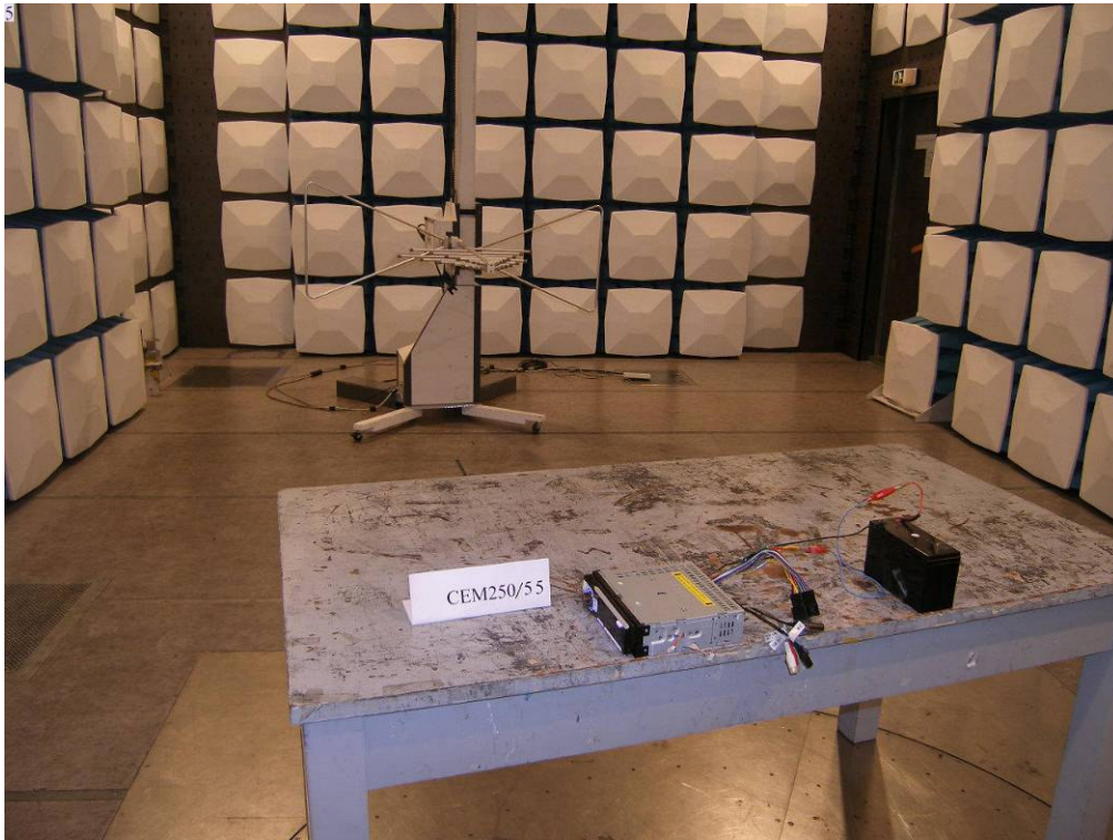
Photograph 1: Set-up for Radiation Measurement below 1GHz
