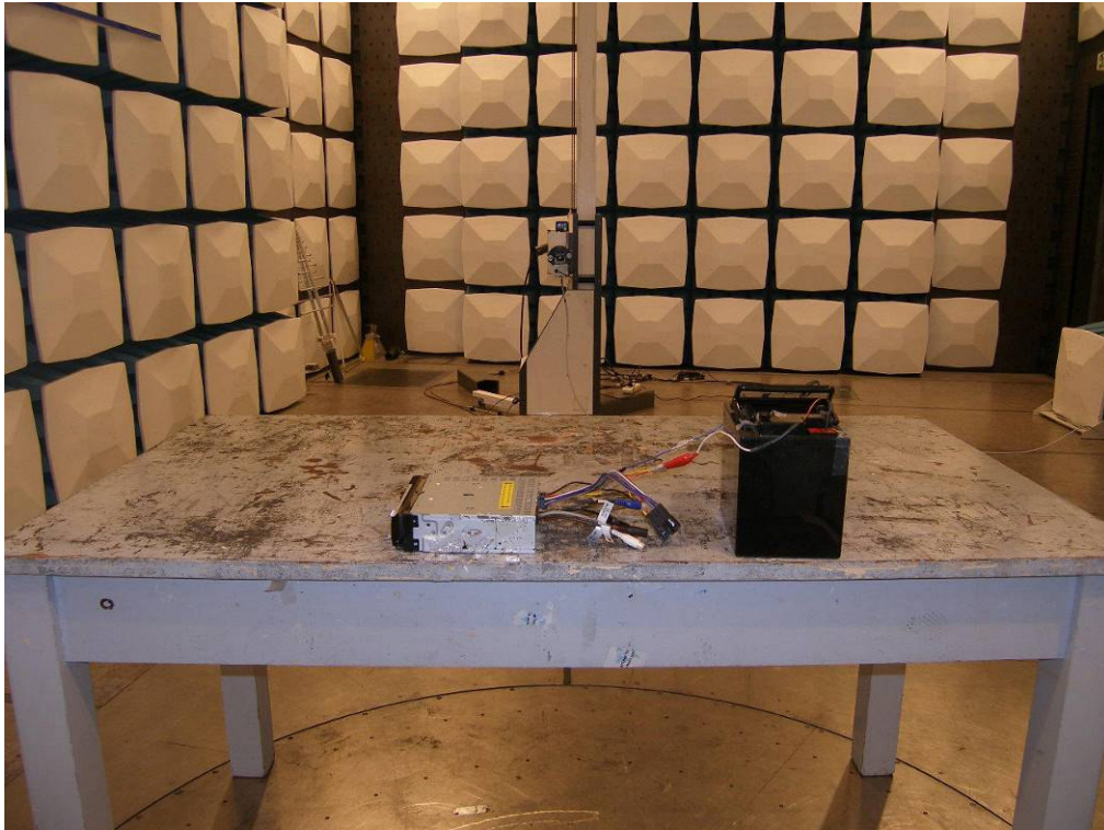
Photograph 3: Set-up for Radiation Measurement 18-25GHz
