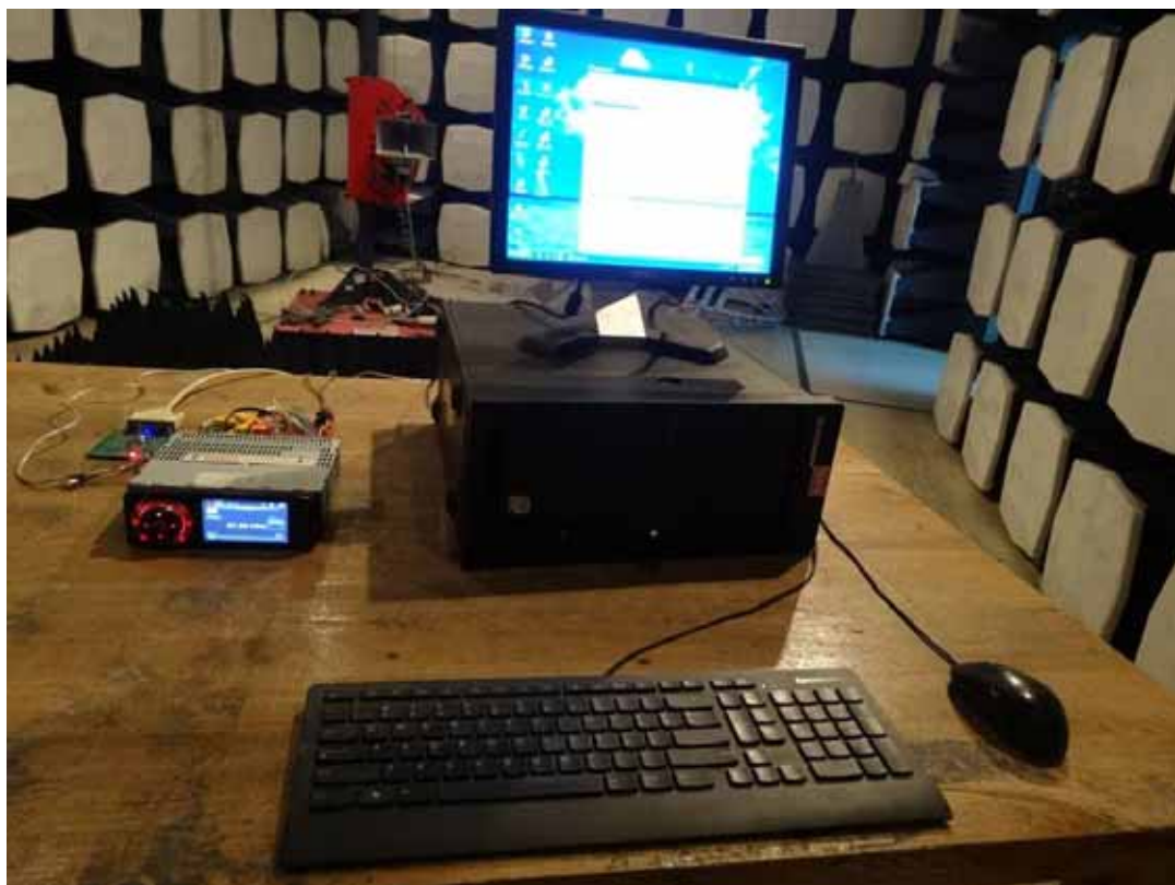
RADIATED SPURIOUS EMISSION TEST ( Above 1GHz )
