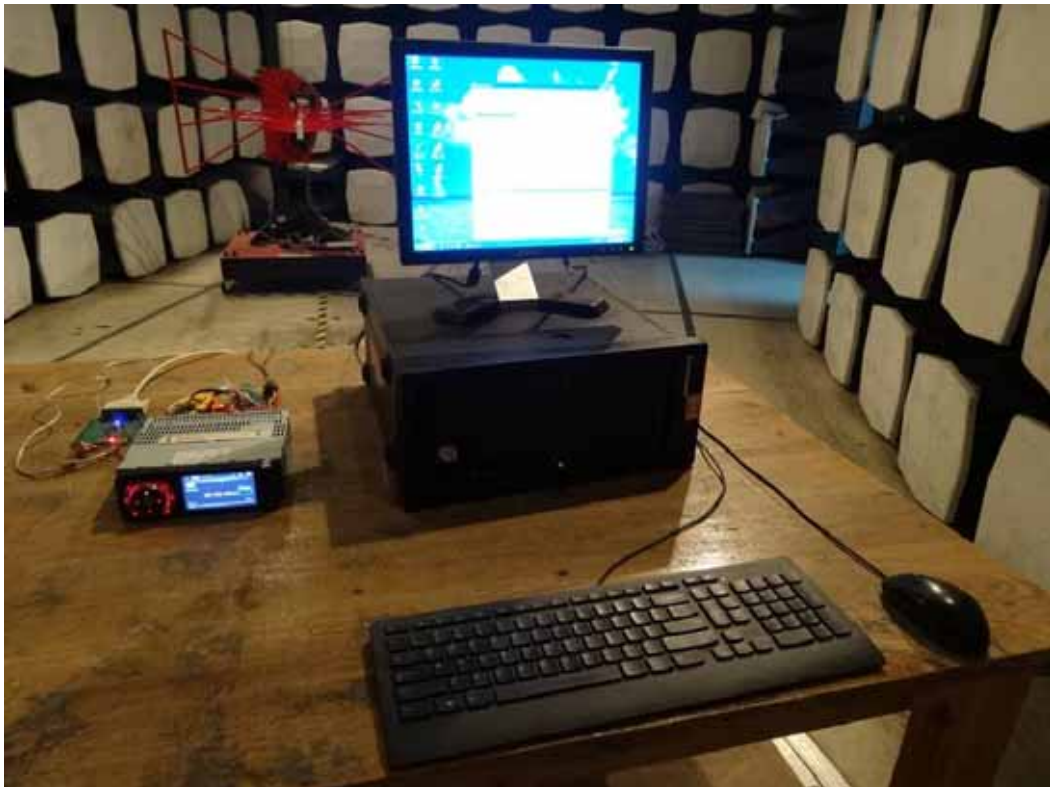
RADIATED SPURIOUS EMISSION TEST ( Below 1GHz )
