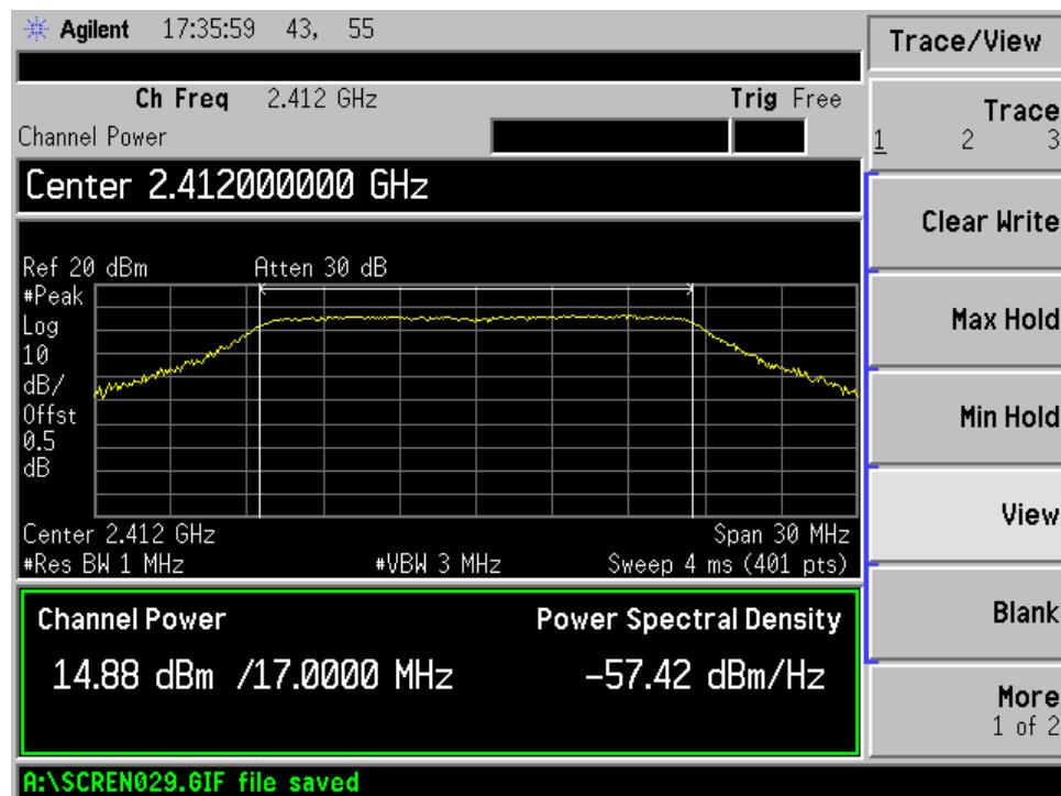
Result data graph shows middle channel conducted power = 14.22dBm
