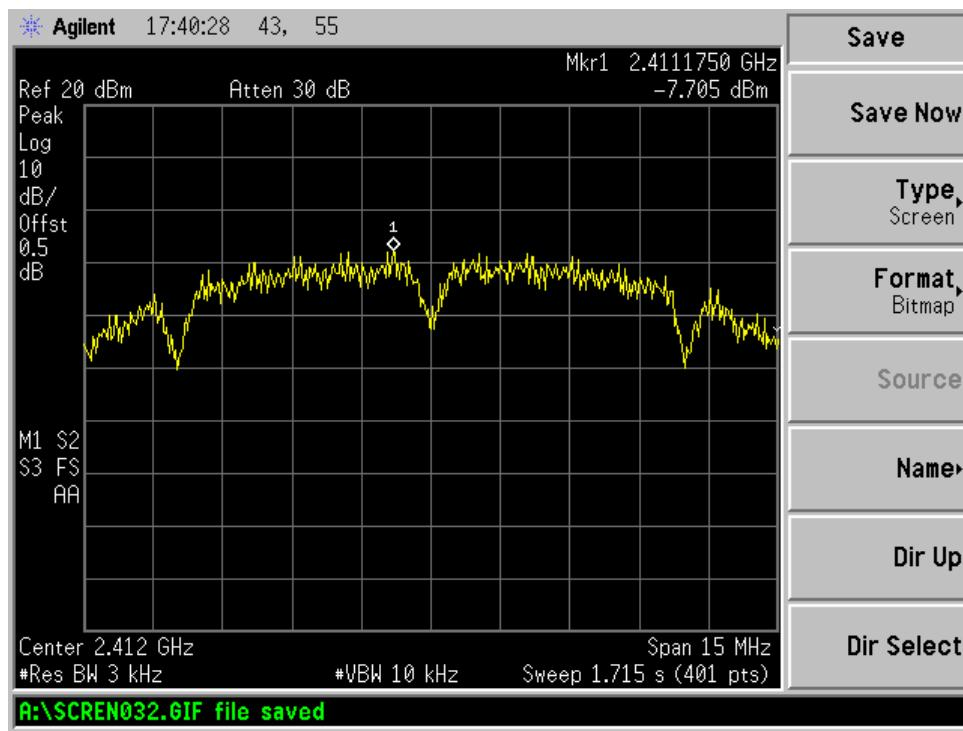
**Result data graph shows middle channel power spectrum density is -8.326dBm at 3 KHz RBW**
