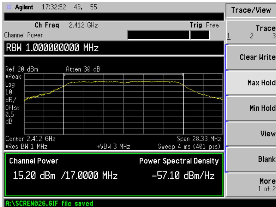
Result data graph shows middle channel conducted power = 15.38dBm
