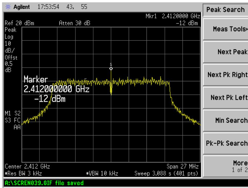
Result data graph shows middle channel power spectrum density is -11.240dBm at 3 kHz RBW
