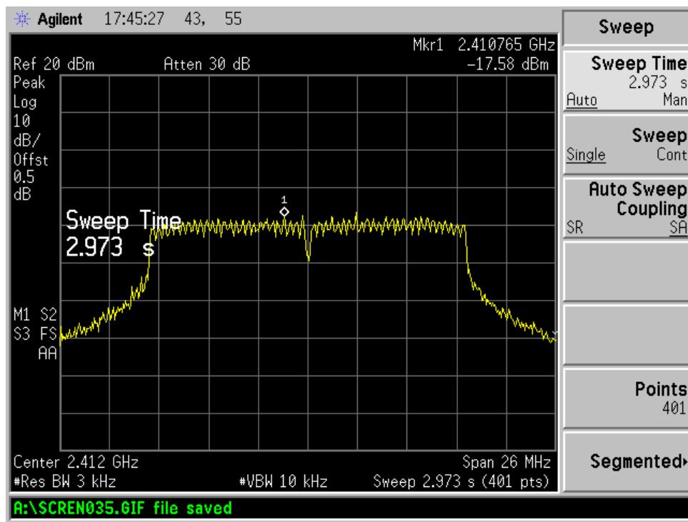
Result data graph shows middle channel power spectrum density is -17.400dBm at 3 KHz RBW
