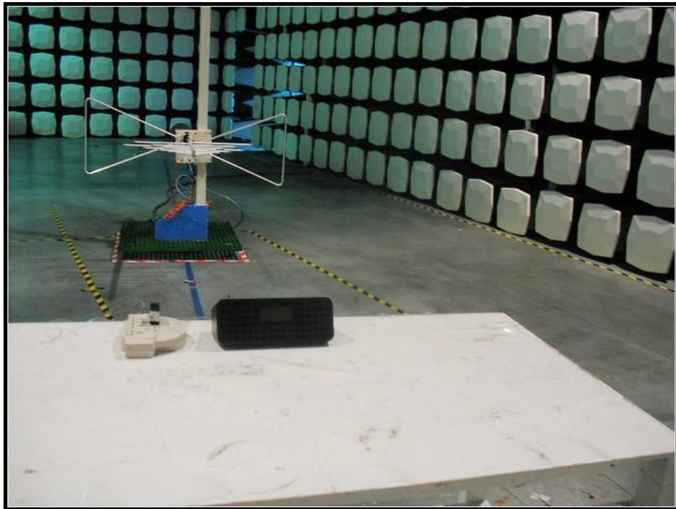
Above 1GHz:(full anechoic chamber)
