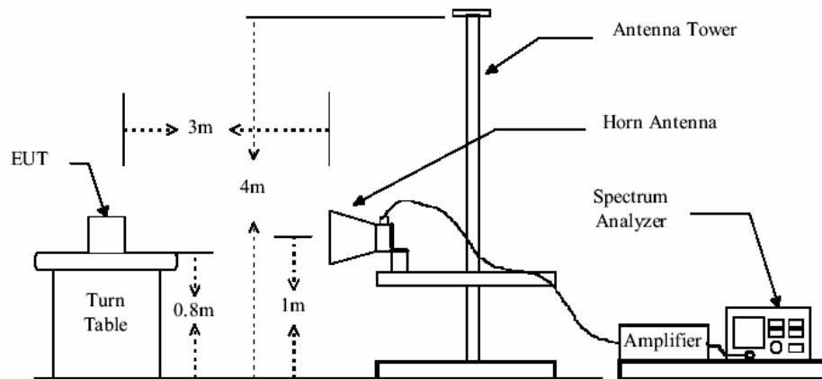
The field strength is calculated by adding the Antenna Factor, Cable Factor & Peramplifier . The basic equation with a sample calculation is as follows:
