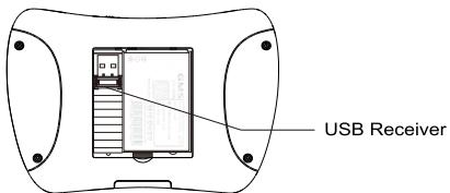
A. Open the battery cover and remove the usb receiver
