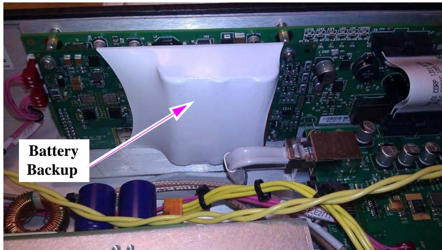
**Figure 5-10 Battery Backup (UPS) Location**
