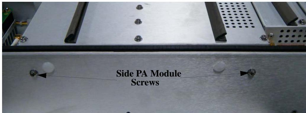
**STEP 5** Loosen the two screws that hold the L brackets to the PA module heat sink and then rotate the L brackets 90° to allow maximum clearance during module removal. (Note: the right bracket may not be used in some versions).
