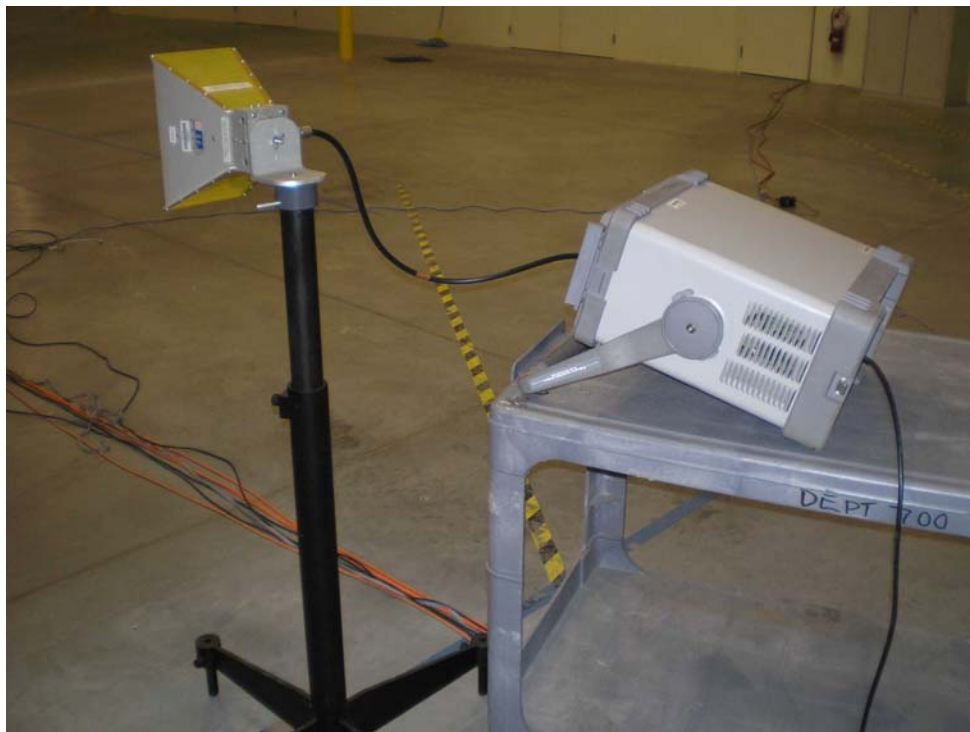
Spectrum Analyzer and Antenna used for these radiation measurements
