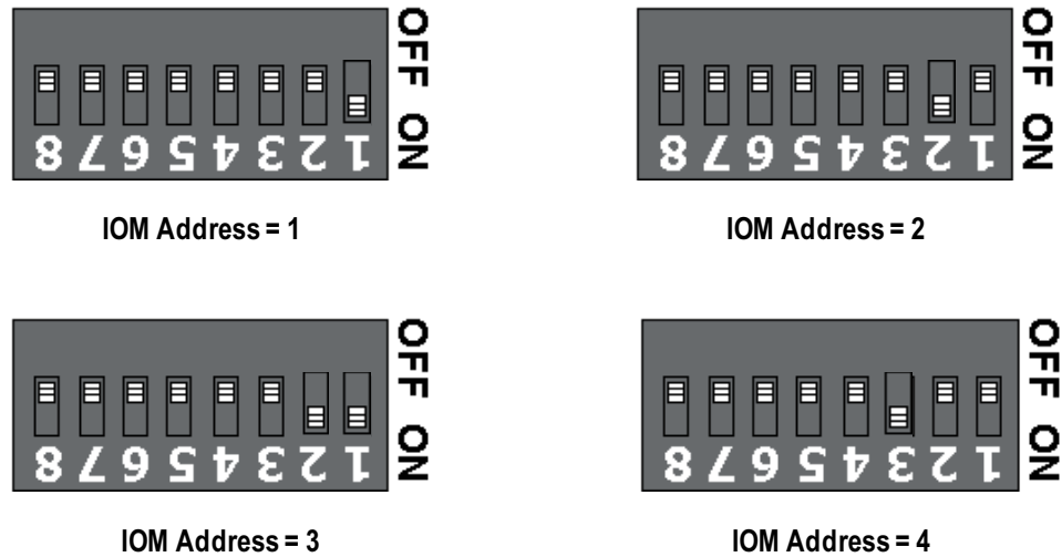
Fig. 32. IOM Address set up - S3 Settings
