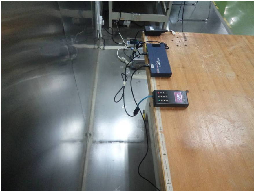
Conducted Emissions - Side View (Powered by PoE)
