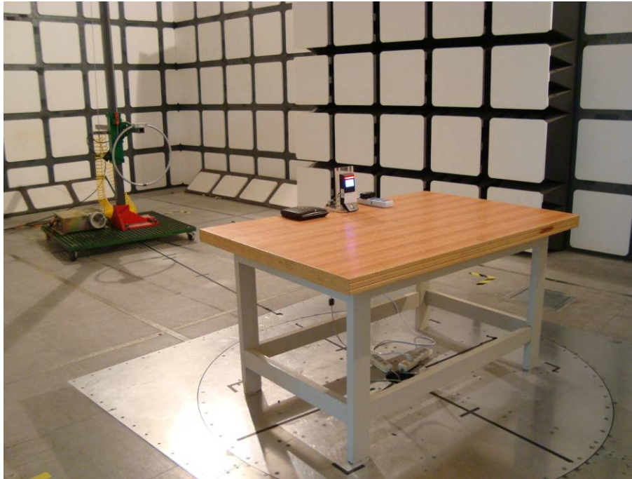
Below 30MHz: Radiated Emissions - Front View (powered by adapter)
