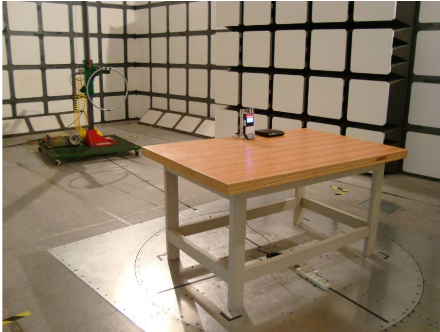
Below 30MHz: Radiated Emissions - Front View (powered by POE)
