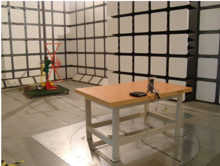
Above 30MHz: Radiated Emissions - Rear View (powered by POE)
