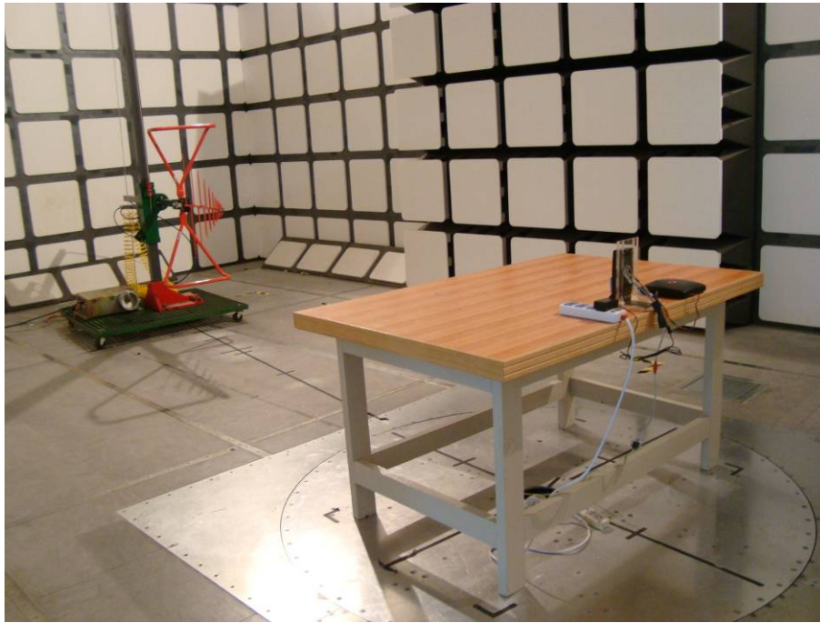
Above 30 MHz: Radiated Emissions - Rear View (powered by adapter)
