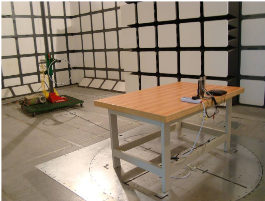
Below 30MHz: Radiated Emissions - Rear View (powered by adapter)
