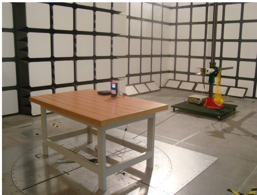
Above 1 GHz: Radiated Emissions - Front View (powered by POE)
