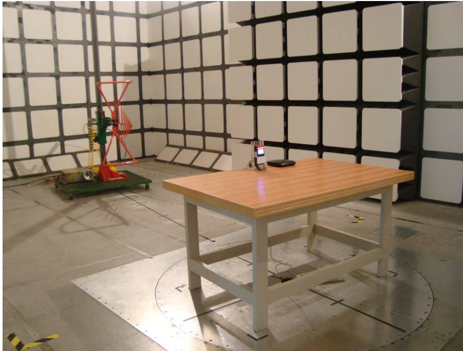
Above 30MHz: Radiated Emissions - Front View (powered by POE)
