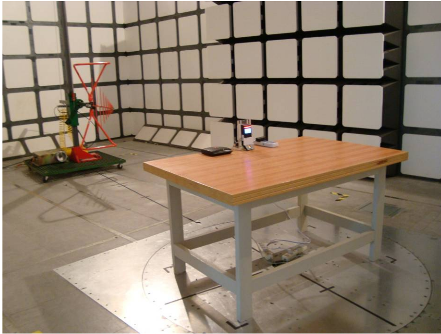
Above 30 MHz: Radiated Emissions - Front View (powered by adapter)
