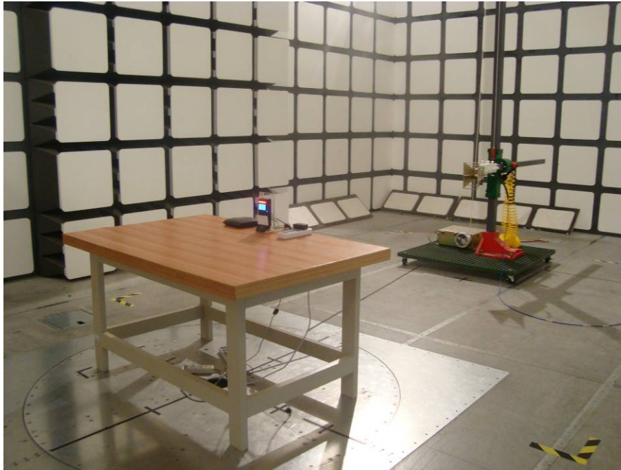
Above 1 GHz: Radiated Emissions - Front View (powered by adapter)
