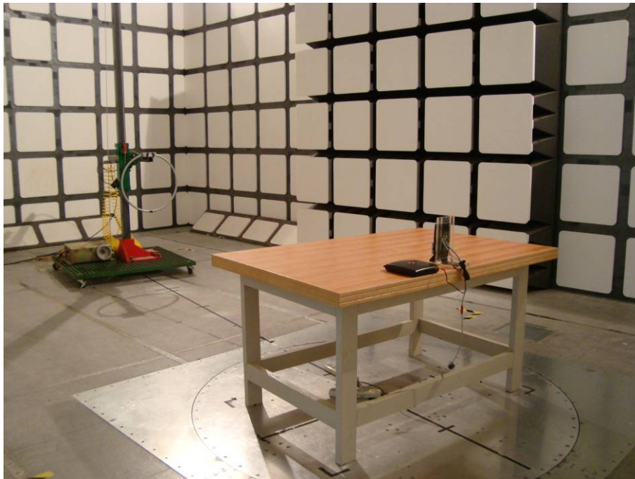
Below 30MHz: Radiated Emissions - Rear View (powered by POE)
