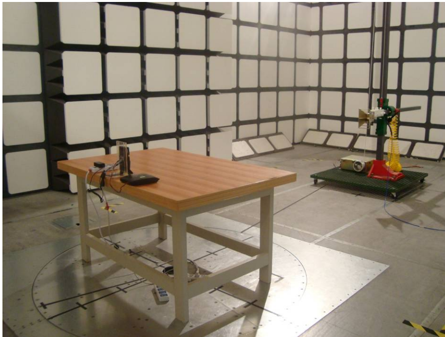
Above 1 GHz: Radiated Emissions - Rear View (powered by adapter)
