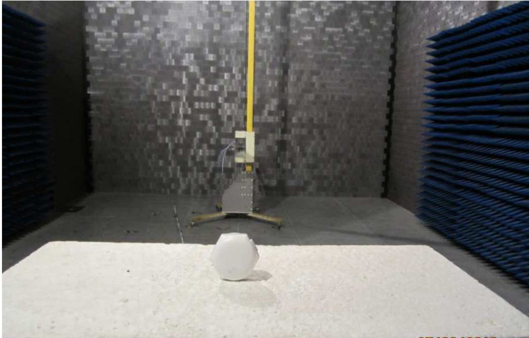
Photograph 3: Set-up for Radiated Emission of Bluetooth, 1G-18GHz
