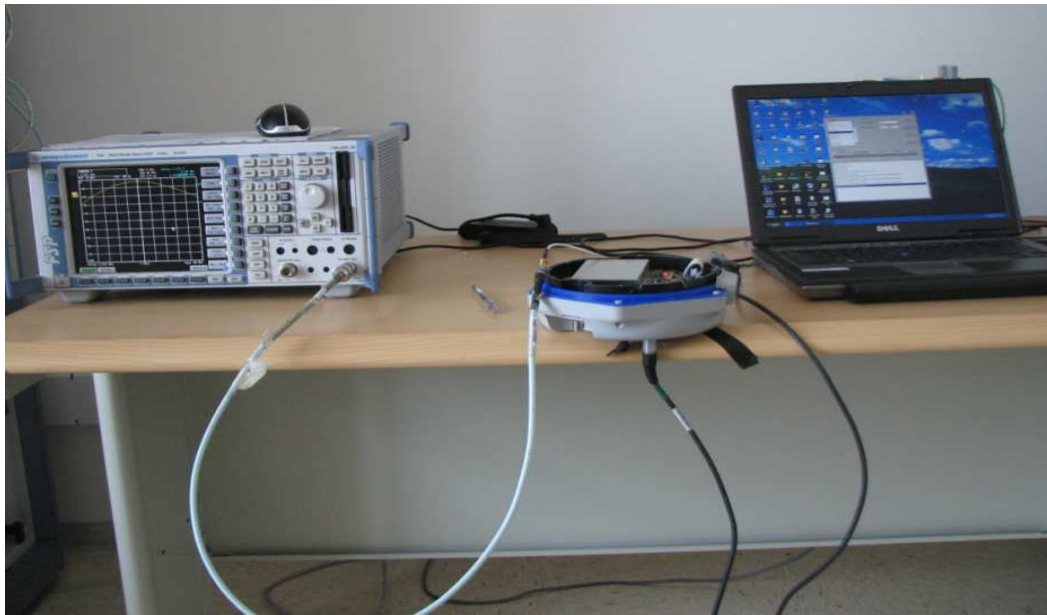
Photograph 1: Set-up for Conducted Emission at Antenna Port
