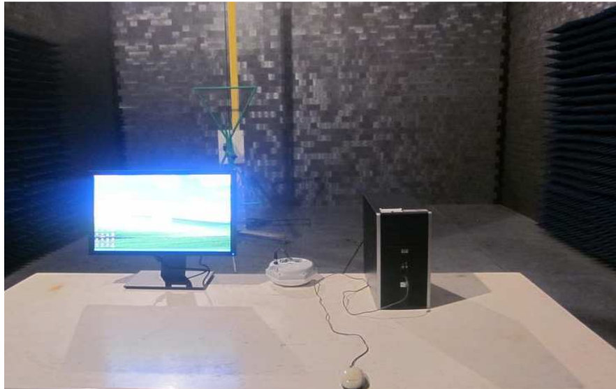
Photograph 6: Set-up for Radiated Emission for Computer peripheral, 30MHZ~1GHZ;
