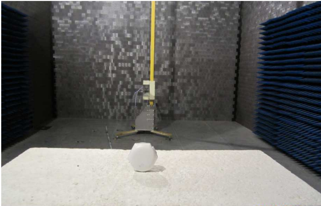
Photograph 3: Set-up for Radiated Emission of Bluetooth, 1G-18GHz
