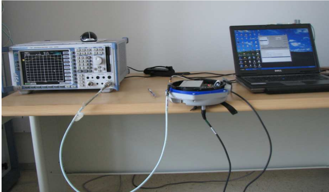
Photograph 1: Set-up for Conducted Emission at Antenna Port
