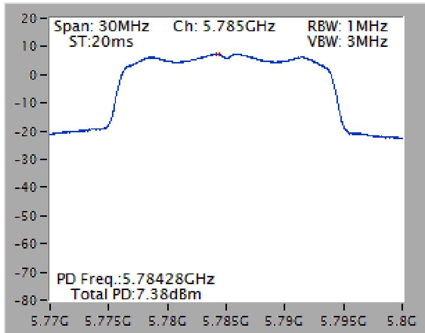
Power Density Plot on Configuration IEEE 802.11n MCS0 HT40 / Chain 1 + Chain 2 / 5230 MHz
