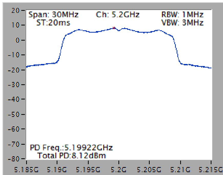
Power Density Plot on Configuration IEEE 802.11n MCS0 HT20 / Chain 1 + Chain 2 / 5300 MHz
