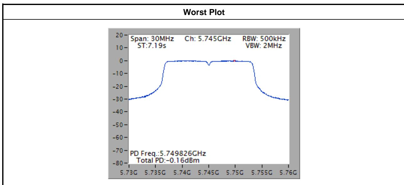
Note: Power Spectral Density plot is without duty factor.
